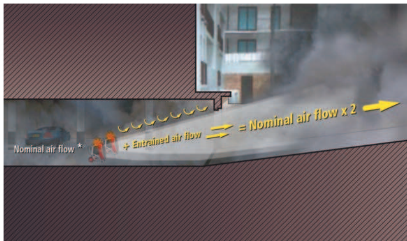
Fig 1 : 2 CarPark Fans in action
